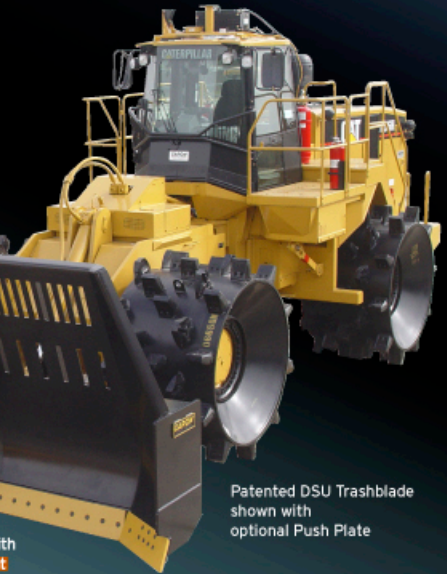
CAT 836H shown with Caron Maximizer® Wheels and patented Caron Double Semi-U® (DSU®) Trashblade
