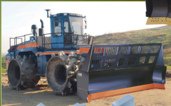
Al-Jon Advantage with Caron MAX® II Wheels and available Caron built Semi-U Trashblade
