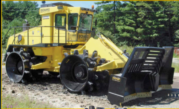
Bomag BC1172RB shown with Caron 8" MegaMax®/BMega Wheels and Caron Double Semi-U Trashblade with Push Plate
